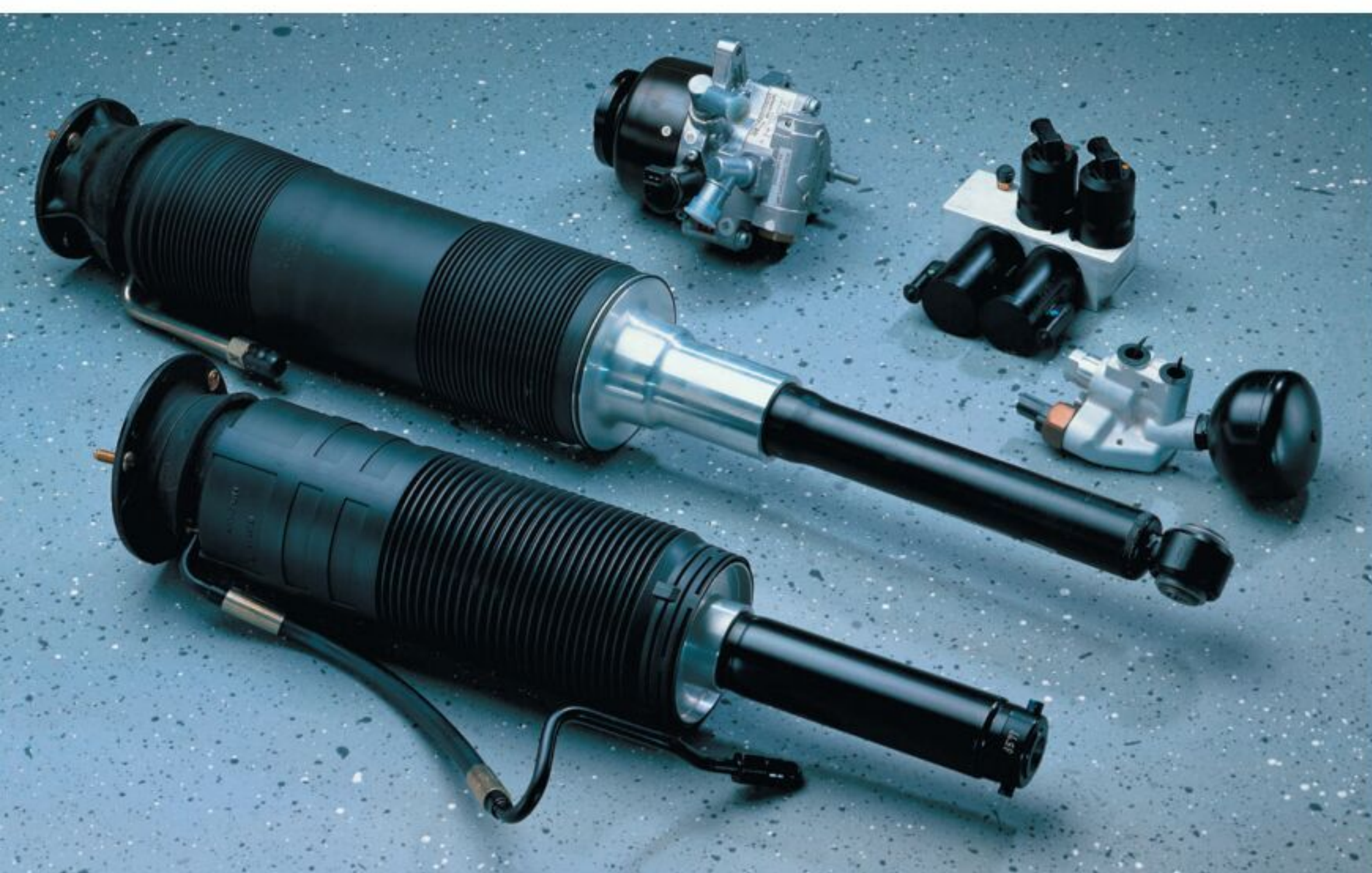
△ Components of Active Body Control suspension set up.
